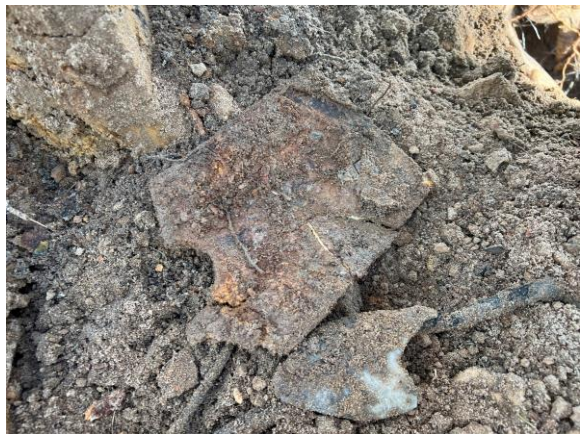
Photo 36: Photograph of asbestos fragment found at TP08-A
