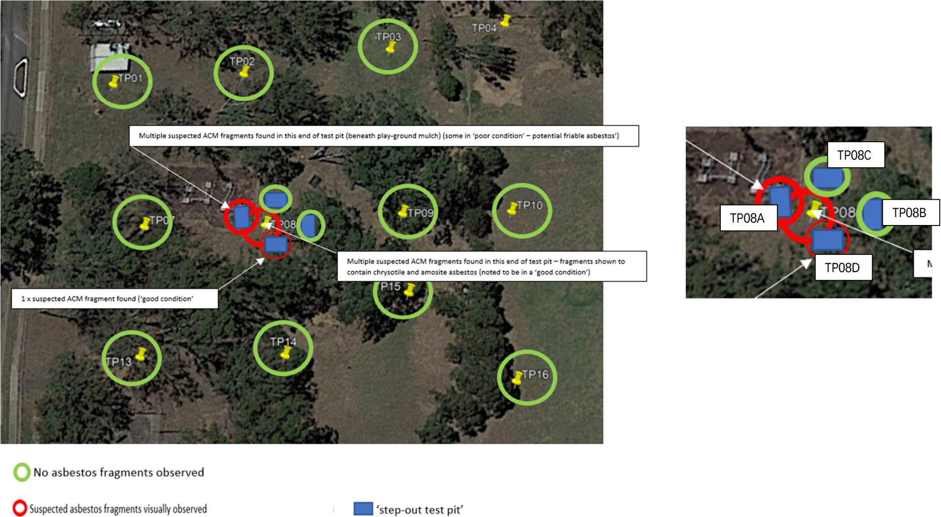
Figure 9-1 – Location of potential ACM finds within TP08 and TP08 series n 'step-out' pits.
