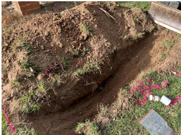
Photo 30: Example of SAND material observed during site investigation
