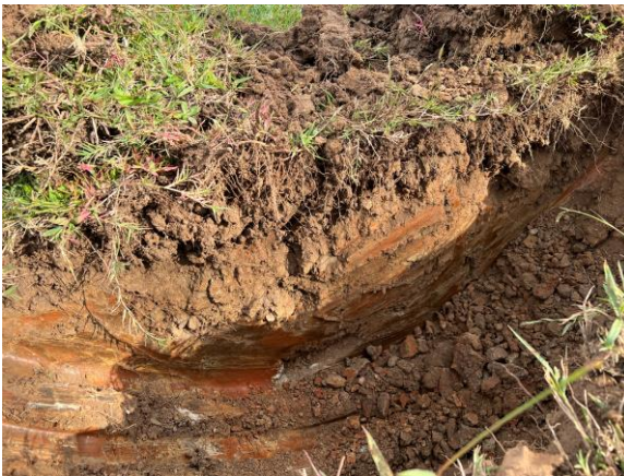
Photo 33: Example of silty CLAY material observed during site investigation
