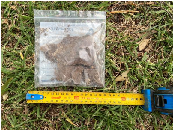
Photo 37: Photograph of asbestos fragment found at TP08
